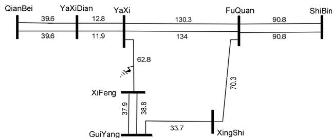
Fig.5. Network topology of the fault area
